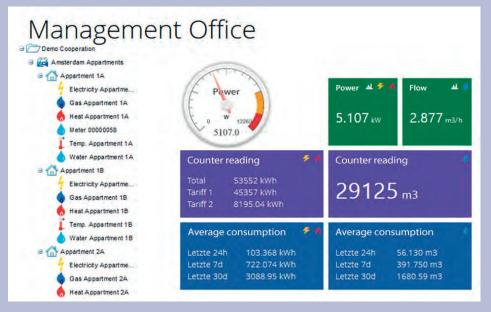
mote measurement of the consumption of electric power and management of public lighting that the PE Roads of Sebia is in charge of. The telemanagement program meant the installation of Wi-Fi devices conducting the measurements and the automatic calculation of the consumption of electric power and on-line remote sending of data to relevant sectors. The alarms set shall send the warnings about non-characteristic consumption of electric power or failure of a part of the system.
