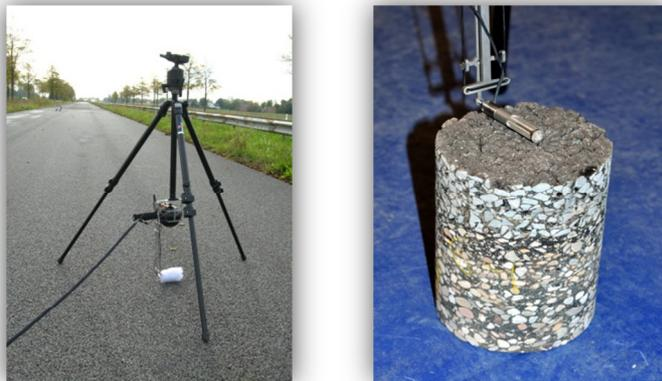
Figure 6: Acoustical impedance measurement on field and on bore cores
