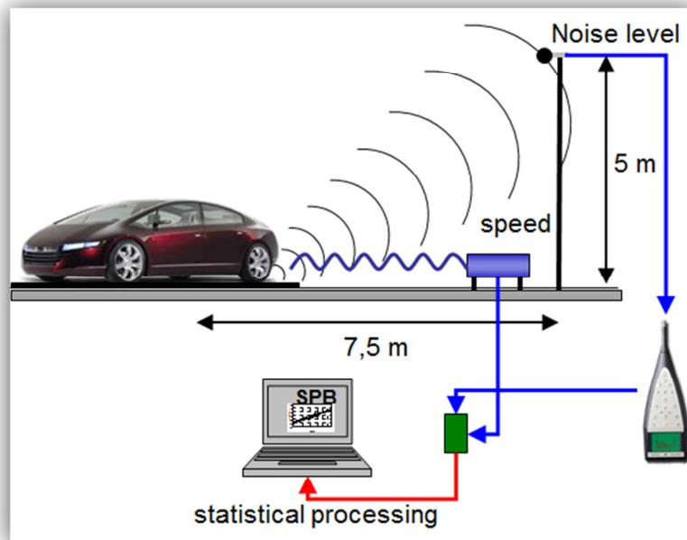
Figure 8: Measurement set-up of the SPB-method.
