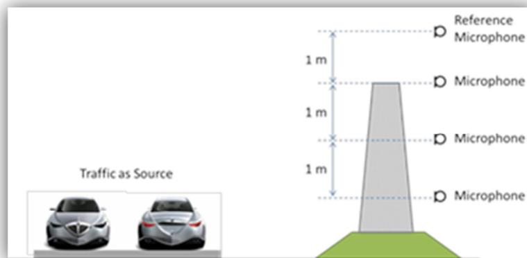
Figure 4: Measurement setup for determine the TL in situ.
