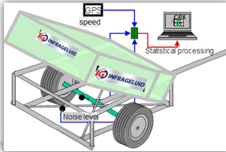
Figure 7: Measurement set-up of the CPX-method.
