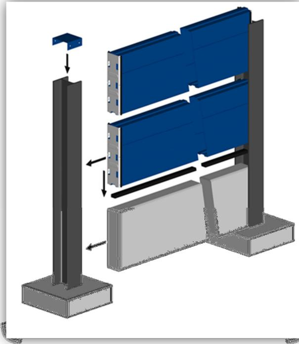
Figure 3: Schematic representation of a barrier made from panels.
