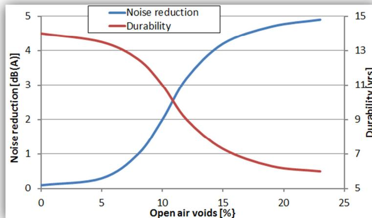
Figure 1: Noise reduction and durability as function of porosity.
