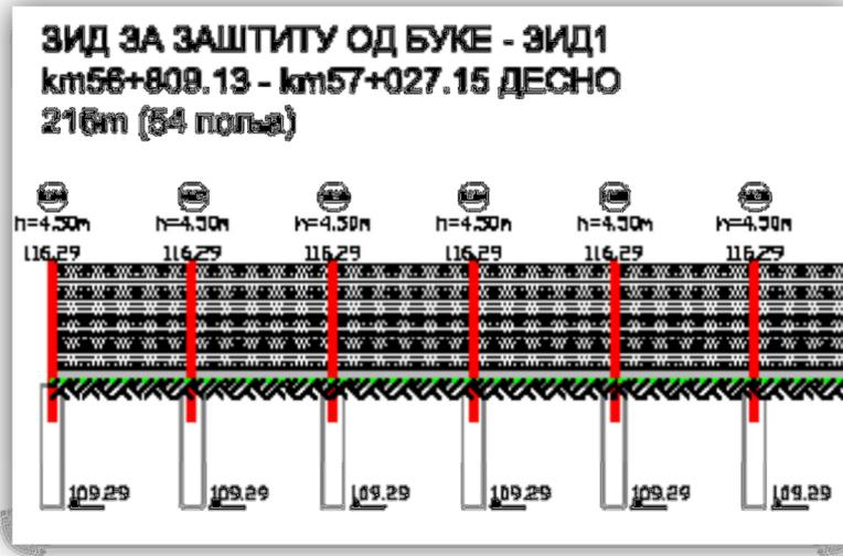
Figure 12: Lay-out of the noise barrier.
