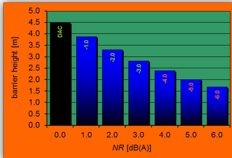
Figure 13: The height of the noise barrier.as function of the noise reduction (NR) of the surface.
