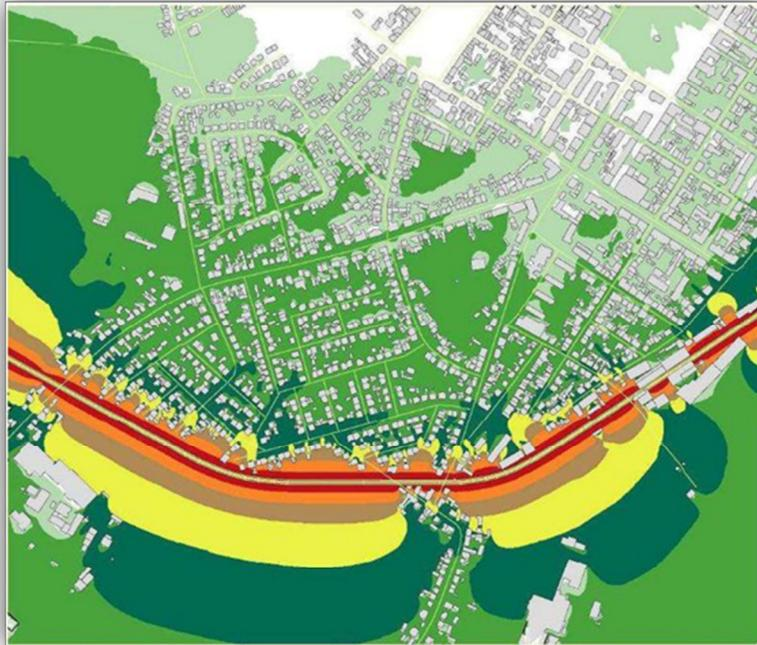
Figure 6: noise contour lines of a case in Serbia.
