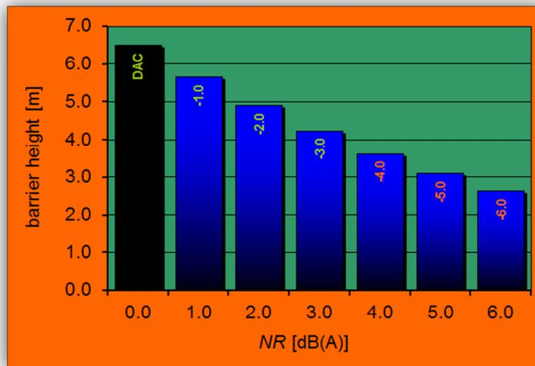
Figure 10: The height of the noise barrier.as function of the noise reduction (NR) of the surface.
