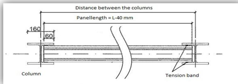
The connection of the panels to the steel posts has to be a click system. The drainage of rainwater requires drainage channels at the ends of the panels. In order to seal properly the elements and the steel posts rubber strips have to be placed on the panels. The rubber has to be 60 ± 5, Shore A.
