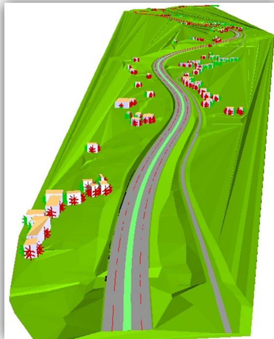
Figure 5: Example of a 3D modelling of a road, its surroundings, and the receivers.
